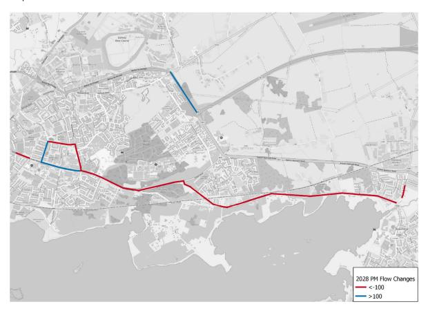
Figure 6-28: Flow Difference on Road Links (Do Minimum vs. Do Something), PM Peak Hour, 2028
