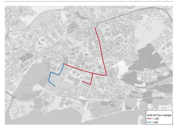
Figure 6-27: Figure 6-27: Flow Difference on Road Links (Do Minimum vs. Do Something), AM Peak Hour, 2028 Opening Year
